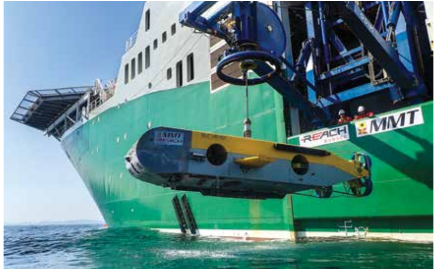
Fig 1. Havila Subsea deploying the SROV Surveyor Interceptor (Joakim Holmlund, MMT, BS MAP)
